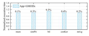
Fig. 15. Performance evaluation of GMODx with five benchmarks which allocate memory using cudaMallocPitch and cudaMallocHost. The performance is the normalized execution time.
