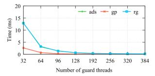
Fig. 11. Average execution time of a guard thread scanning its byte array for once.
