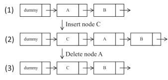
Fig. 7. List structure. From (1) to (2), node C is inserted into the list; and from (2) to (3), node A is deleted from the list only if node A is not the next node of the dummy node.
