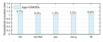
Fig. 14. Performance evaluation of GMODx with five benchmarks. The performance is normalized by the execution time of applications without GMODx.
