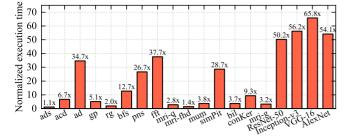
Fig. 18. Performance evaluation of cuda-memcheck. Performance is normalized by the execution time when overflow detection is disabled.
