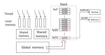
Fig. 2. Illustration of stack overflow.
